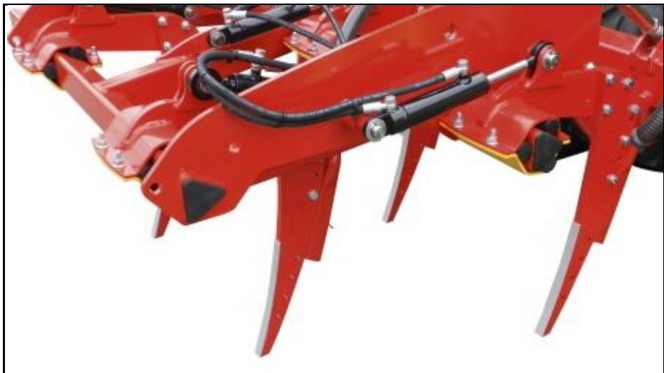
Figure 11: Example of a strip till drill
